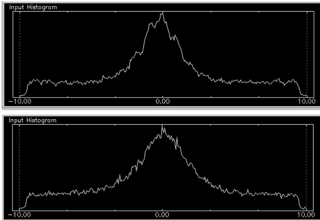
Figure 2: Orbit 2037: Correlation results (1: line shift, 2: column shift) obtained between SCARAB and SAPHIR product computed with calibrated parameters.
